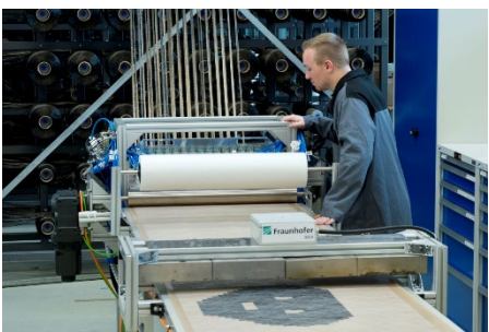
Image 3: Continuous Fiber Tailoring (CFT) is a highly efficient process developed by Fraunhofer IGCV: near-net-shape carbon fiber preforms used to manufacture CFRP components can be produced automatically using this process. | Copyright: Fraunhofer IGCV
