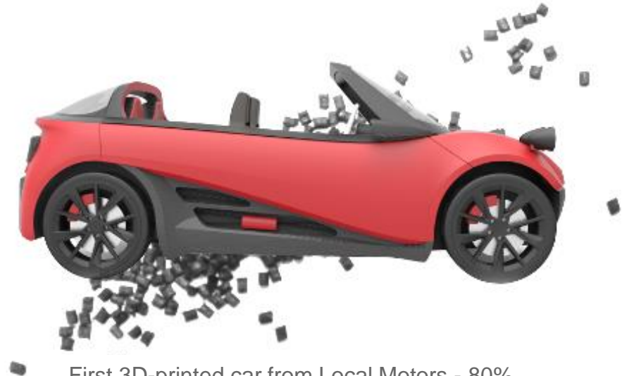
First 3D-printed car from Local Motors - 80% ABS plastic and 20% CF
