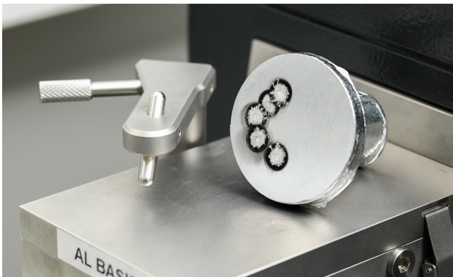
Melting analysis with an emission spectrometer
